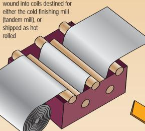
and pickled. In either case, a surface and/or edge treatment of the coil with oil or water based **VpCI**™ products is recommended.
